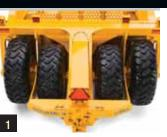
Staggered wheel pattern is self-cleaning and increases floatation for high-speed finishing and easier pulling in muddy conditions. Provides more stability, too.
