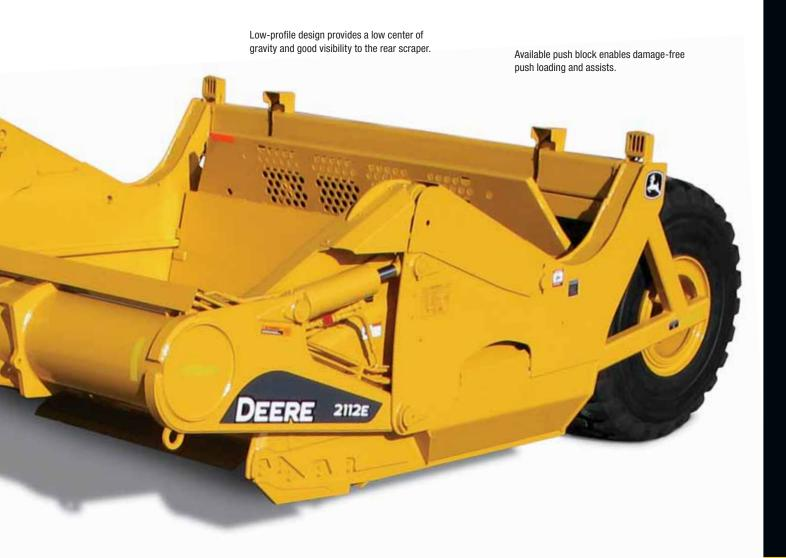
Two rows of bolts and six-inch spacing let you mix and match standard and long blades in a variety of configurations to fit almost any application or material condition.
