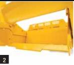
2. Wide 55-inch throat opening allows quick and easy loading and dumping, and lets you handle a wide range of materials.
