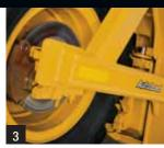
3. Need more stopping power? Equip your 18- or 21-cubicyard scrapers with optional heavy-duty disc brakes. For shorter stops, loaded or empty.
