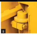
Ejector wall rollers are positioned where they're protected and are adjustable to maintain ejector, sidewall, and floor clearances.
